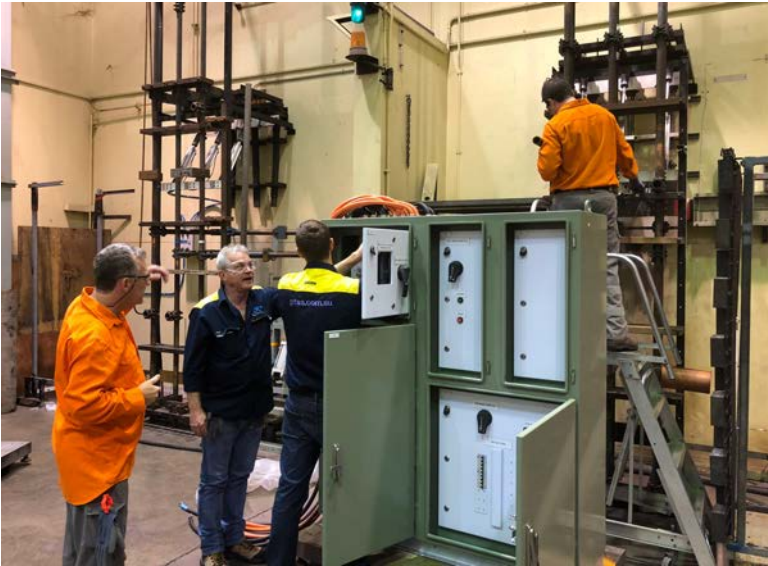
NATA Certification Testing of the Arc Blast Containment & Diffusion (ABCD) compact modular outdoor switchboard. PTAS 'Switchboard-Online' (QR Code)
