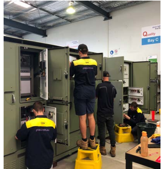
A wide range of indoor and outdoor electrical controls switchboards are designed, fabricated and manufactured in-house
