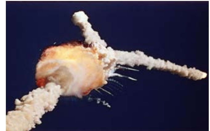
NASA Challenger failure was more than the physical 'o-ring failure'; crossing the jet stream + public pressure to launch + oscillation of booster
