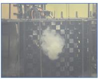
hazards. By being engineered and physically tested to contain an arc fault whilst maintaining structural integrity, the risk to operators and bystanders has been minimised without the reliance on a device operation.
